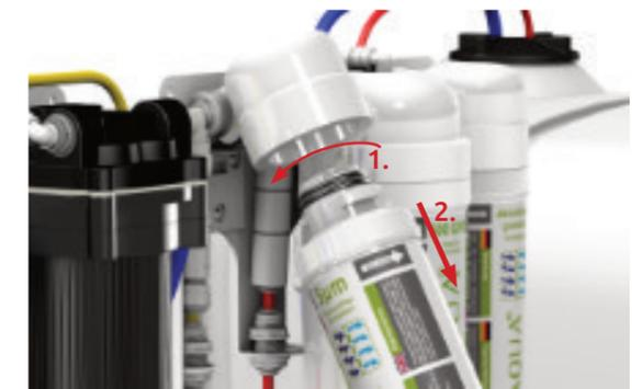
Turn the filter cartridges outerclockwise 90° out of the filter heads to change the filter units.
